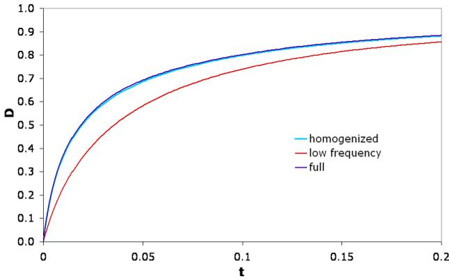
Fig. 3 Damage  $D$  evolution far from the elliptic hole (zoom)
