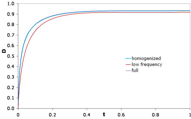
Fig. 2 Damage  $D$  evolution far from the elliptic hole
