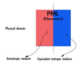
Figure 5: Schematic presentation of the introduction of the isotropic equivalent material in the PML.
