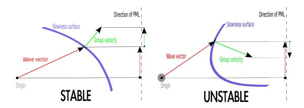
Figure 4: Instability issue with PMLs in anisotropic medium.
