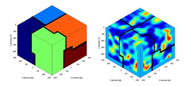
Figure 3: Example of fields generated by sub-domains (one sub-domain per thread): geometry of the sub-domains (left figure) and one realization of the component  $C_{44}$  of the elasticity tensor (right figure).
