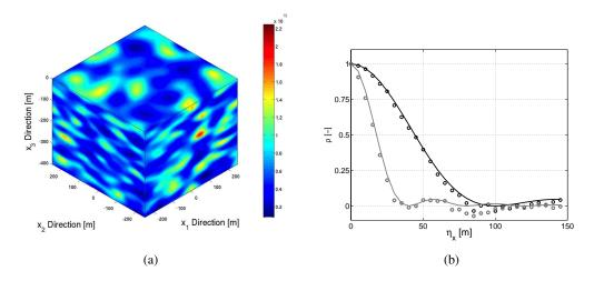
Figure 1: A sample of stochastic elasticity tensor field: (a) Mapping of  $C_{11}$ . (b) Theoretical (solid lines) and observed (circles) correlation structures in  $i_1$  – (black) and  $i_3$  – (gray) directions.
