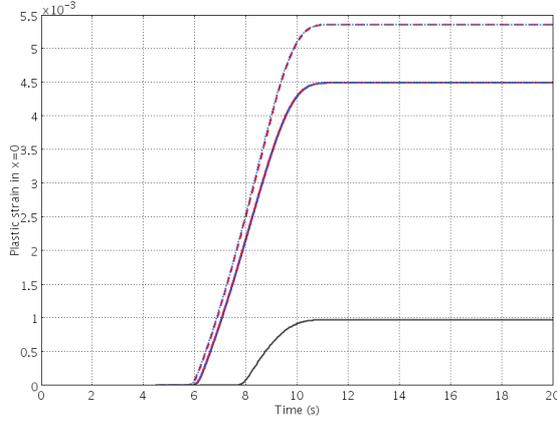
**Figure 2.** Plastic strain in  $x = 0$ : reference solutions (in red) and time-homogenized (in blue) solutions (dynamic and quasistatic); quasistatic solution when the fast cycles are not taken into account in the homogenization process (in black).
